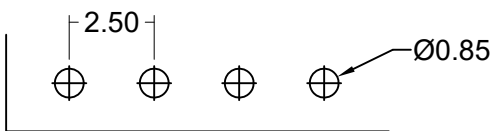
Recommended P.C.B Layout General Tolerance \pm 0.05
